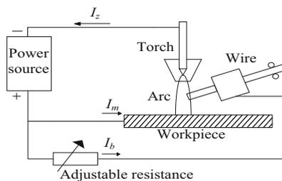
**Fig. 1.** Principle of bypass coupling micro plasma welding
