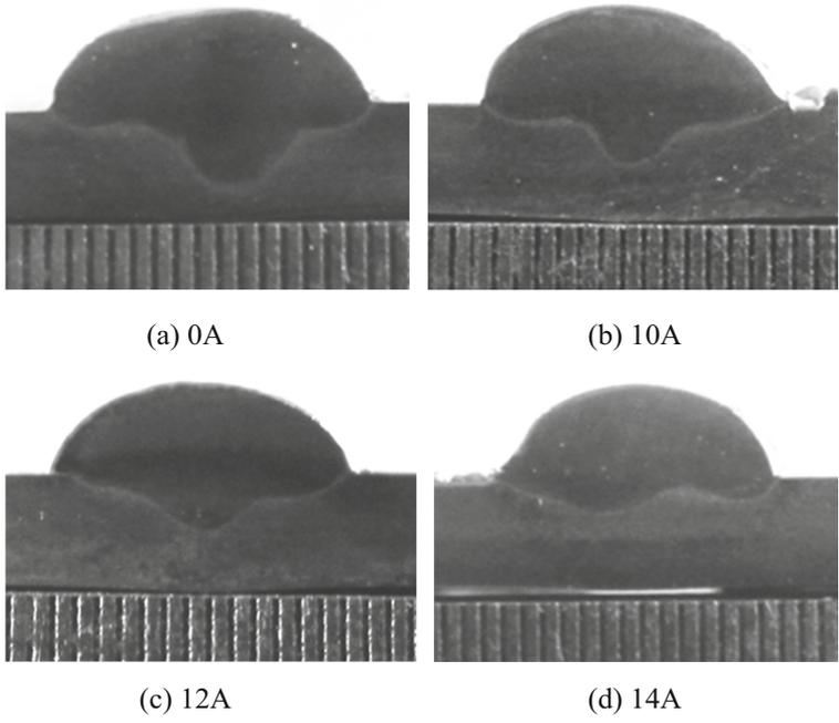
**Fig. 6.** Transverse of welding seams at different bypass currents
