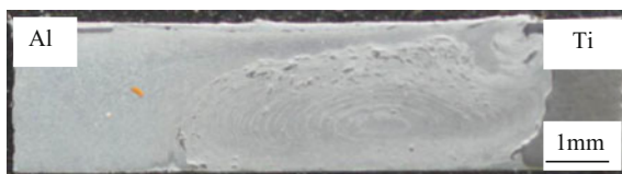
Fig. 3 Cross-section structure of dissimilar joint prepared by FSW
