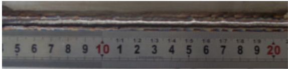
(o) welded seam formed during test 15
