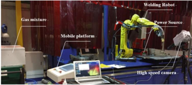
(a) Experimental set-up for welding and observation
