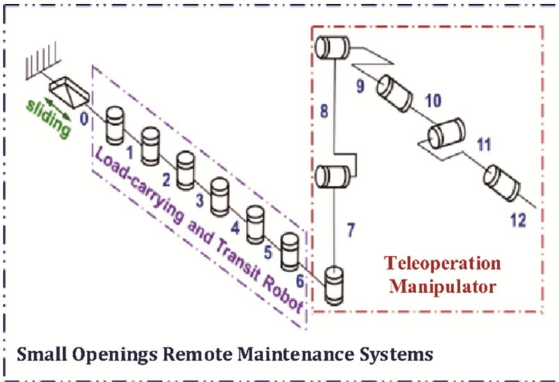
Fig. 2. The configuration of the 12-DOFs manipulator
